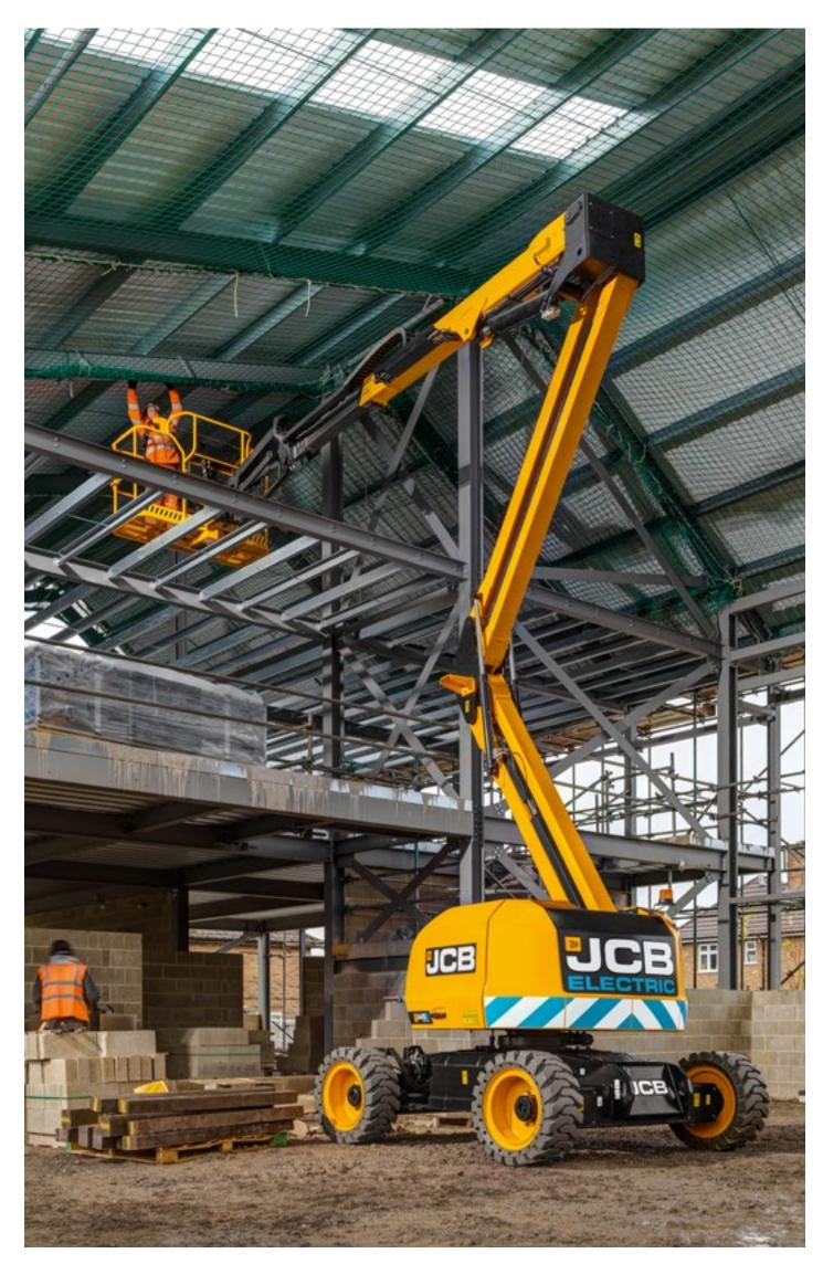
Rechargeable batteries alongside the JCB Diesel by Kohler engine allow for an extended standalone run time.
